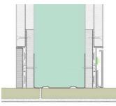
Example skirting board mounted on double sheet plasterboard, base item no. 88/6 + inserts.
