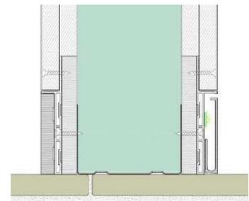
Example skirting board mounted on double sheet plasterboard, base item no. 88/6 + inserts.
