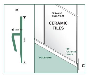
Capping strip gives a neat finish to the installation and ensures a continuous, sealed surface.
