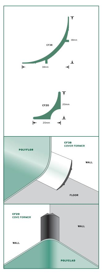
Where ease of maintenance and hygiene are important, sheet flooring may be taken up the wall having created a radius using our Cove Former.
