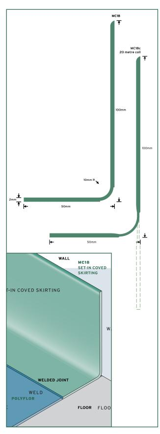
Skirting of this type is fitted before the flooring is laid, where a simple butt joint is required. Welded to the flooring, this provides a secure joint.
